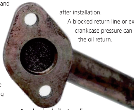
A carbonised oil return line may cause a replacement turbo to fail
