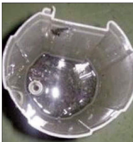
Paint sludge inside the fuel pump assembly
