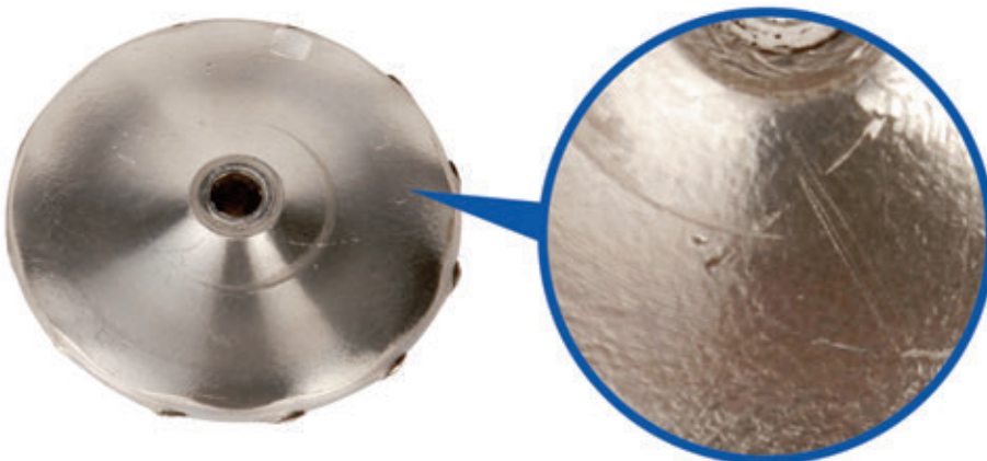
Orange peel on the back of the inducer is another sign of overspeeding
