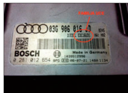
The ECU type can be read off the label
