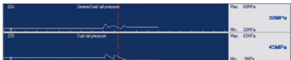
Figure 2 - The actual fuel pressure sometimes exceeded the desired fuel pressure
